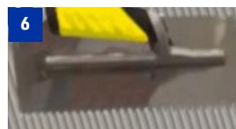
6 Trowel required to adhere mat: **4.5mm x 4.5mm** square notch, or **3/16" x 3/16"** square notch.
