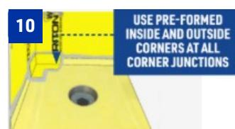
Ensure that all seams have a min. 2" overlap of Triton Waterproof Membrane fabric or Seam Tape adhered with mortar.
