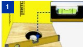
Prior to installation of Triton Pre-Sloped Shower Pan, floor must be level and traditional clamping drain must be properly installed.
