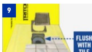
Apply Triton Adhesive Sealant to four corners of plastic grate holder prior to fitting grate tray.
