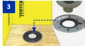
Attach adaptive drain base using the 4 bolts from step 2.
