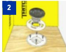
Remove 4 drain base bolts, locking collar, and adjustable drain barrel.
