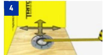
To cut Pre-Sloped Shower Pan, measure from drain center to each edge.
